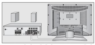
Connect the white and red sockets »AV OUT L R « on the television and the corresponding sockets on the HiFi with a cinch cable.
